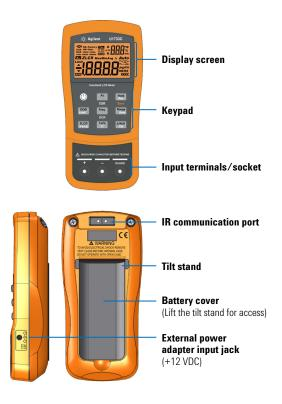
The external AC to DC power adapter input jack requires an input voltage of +12 VDC.
